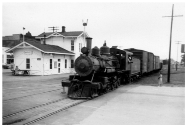
This southeast Georgia short line is the Louisville & Wadley and their 4-6-0 #42 has stopped at their Wadley depot with its mixed train. Wadley was an early capital of Georgia. This 10 mile line was also owned by the Central of Georgia. It was sold in 1961 and was abandoned by 1971. The L&W interchanged with the C of G and the Wadley Southern in Wadley. - Lakeland Public Library, Sanborn collection
