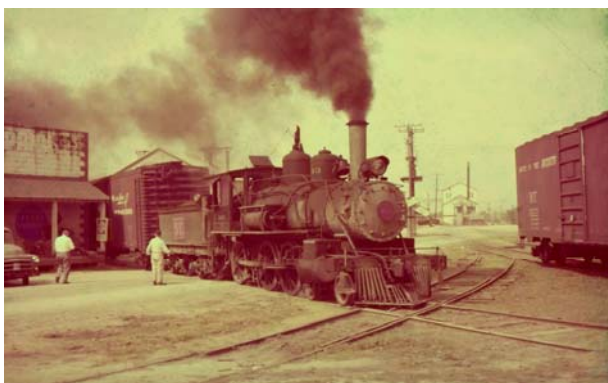
This month takes us to several very colorful Georgia short lines, all photographed by the Sanborn brothers of Lakeland, about 1950. This photo captures Sylvania Central 4-6-0 #103 spotting cars at customer's sidings in Sylvania in southeast Georgia. This 15 mile line, from Sylvania to Rocky Ford, was controlled by the Central of Georgia and was abandoned in 1954. - Lakeland Public Library, Sanborn collection
