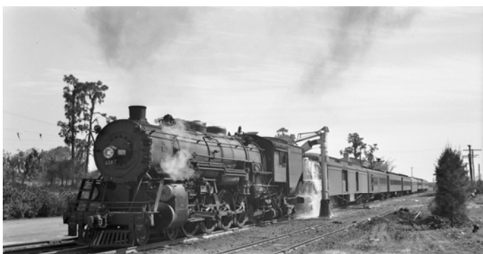
This scene finds SAL 4-8-2 219, class M-1, taking water while making a north bound stop at Sebring, Florida in the early 1940s, as it made its way from Miami to New York City. The second car is an RPO-coach and the fifth car an SAL " American Flyer " car, nick-named due to its design looking similar to cars produced by the toy train maker with that name. Sam Appleby photo, CFRHS collection
