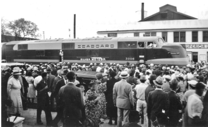
This photo of SAL's new EMC E4 3006 as it arrived in St. Petersburg, Florida after pulling the very first Silver Meteor from New York City on February 7, 1939. This new all stainless steel streamliner drew a large crowd of spectators, which is evident in this scene. The Silver Meteor name plate on the locomotive would eventually be removed to allow more flexibility in power assignments. Sam Appleby photo, CFRHS collection
