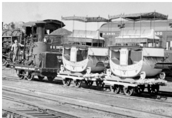
The B&O's Atlantic , nicknamed a grasshopper due to its horizontal beams and long connecting rods, was built in B&O's St. Clair Shops in 1832. It weighed in at 6.5 tons and had a T.E. of 4,245 pounds. It was scrapped in 1835. A similar engine named the Andrew Jackson , built in 1836, was modified to be the 1832 Atlantic , and it was first exhibited in 1893. It is now preserved in the B&O Museum. – CFRHS collection
