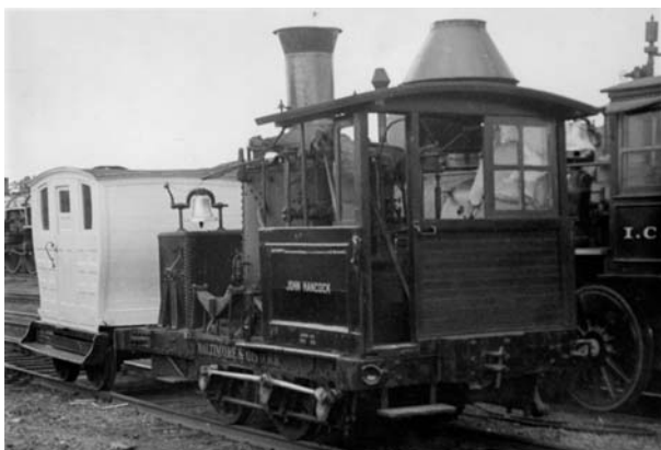
B&O's John Hancock , also a grasshopper type, was built in the B&O's St. Clair Shops in 1836. The 0-4-0 weighed in at 14.5 tons and had a T.E. of 5,094 pounds. It was B&O's first to have roof over the cab and all 4 wheels powered. In the 1850s it became known as #8 when the B&O ceased naming their locomotives. It was in continuous service until 1892 when it was retired. It now resides in the B&O Museum. – CFRHS
