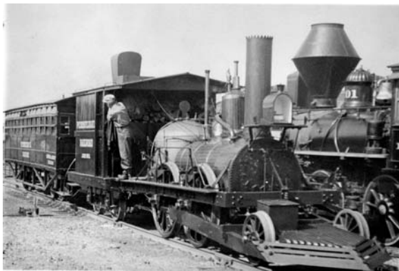
The late John Rapalje, a longtime member, attended the Chicago RR Fair of 1948-49 and took these 3 photos. This one is the John Bull replica built by the Pennsylvania RR in 1939 to promote progress. The original 2-4-0 was built in England and first operated on the Camden & Amboy in New Jersey in 1831. This line became part of the PRR and the original John Bull was sold to the Smithsonian in 1884. The replica is now preserved in the RR Museum of Pennsylvania. – CFRHS collection
