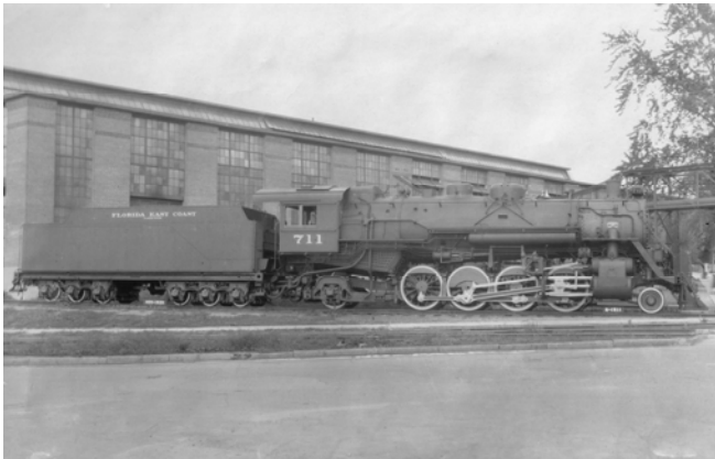
The FEC had 15 of these 2-8-2 oil burning, steam locomotives built by Alco in 1925. Number 711 is an example of these powerful freight haulers that shared that duty with the 23, 800 class, 4-8-2s, that could also handle heavy passenger trains, and 15, 300 class, low-driver, 4-8-2s. All of these Mikados remained on the roster until 1955 with one leaving in late 1954. CFRHS photo
