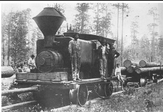
Logging RR with pole rails and a steam traction engine for motive power. Photo courtesy of ACL-SAL Historical Society.
