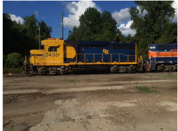
Started out life as ATSF 1235 then became 3235 in the '69-'70 general re-numbering. It was rebuilt in kind as a GP-30u in the early 80s to the 2735 then became BNSF 2435 in the merger. LTEX stands for Larry's Truck & Electric Co. , a locomotive lesser.
