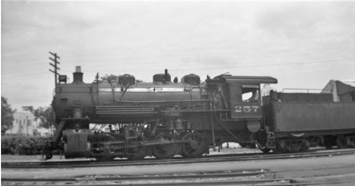
FEC's modern steam switchers were all Alco built, oil burning, 0-6-0s and 0-8-0s. This photo of 0-8-0 #257 in Miami in 1941 is one of 29 locomotives of this class built between 1924 and 1926. Twelve stayed on the roster until 1954 and 55. Number 253, presently being restored in Ft. Pierce, was sold to the Louisiana & Arkansas RR in 1936, which led to it being saved as a park display in 1956 in Texarkana, TX. CFRHS
