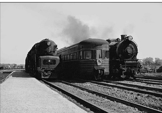
At Englewood Union Station on the South Side of Chicago, Pennsylvania Railroad T1 4-4-4 -4 5514 and M1 4-8-2 6975 bracket the observation car of the Trail Blazer , which is just pulling out for New York on a July 1947 afternoon. Thanks to Society Member Roger Wilson for this Milton B. Nafus photo.
