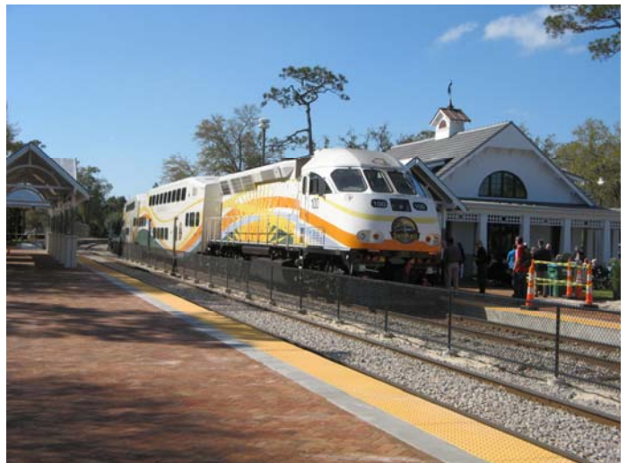
SunRail's display train at Winter Park's new depot dedication had two coaches, the last one being a cab control car. SunRail's standard seems to be the cab control car in the lead south bound and the locomotive in the lead north bound.
