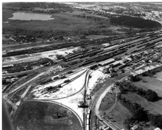
This aerial of the ACL's Lakeland shops and yard was taken in the mid to late 1950s, soon after dieselization was completed. The freshly cleared soil is where the turntable and roundhouse were located. They have been replaced by a locomotive turning wye and a run-thru engine shop. The water tank in the lower center was kept for filling boiler water tanks on passenger diesels. - Dick Kearns collection
