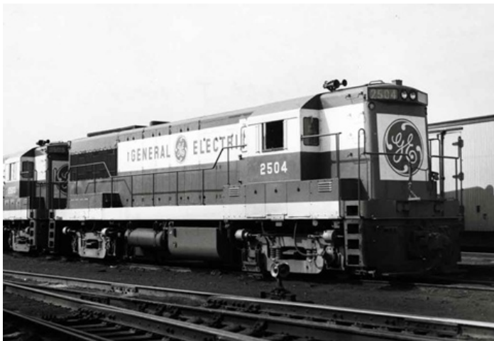
General Electric 2504 was part of a set of four red-and-white U25B demonstrators the builder fielded in 1961–62. GE 2501 had a low nose, while 2502–2504 had high noses, which were passing from favor at the time. J. David Ingles photo.
