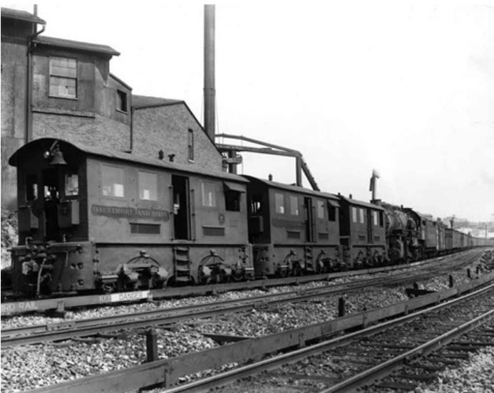
Three Baltimore & Ohio box-cab electric locomotives help a Mikado-powered freight on the Baltimore Belt Line. Four of these ungainly motors replaced the Belt Line's original steeple-cabs in 1903. Unusually, the box-cabs' four powered axles were rigidly mounted in the frame, giving them an 0-D-0 wheel arrangement. B&O photo.
