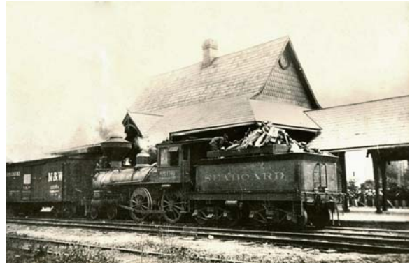
This April 1, 1914 scene is of Seaboard Air Line's depot on the north side of W. Central Ave. in Orlando. The depot was built to identical plans of SAL's Ocala depot. SAL 4-4-0 #506 had a full load of wood as it tended to its local switching duties. - Donated by Claude Hunter, SAL's freight agent.
