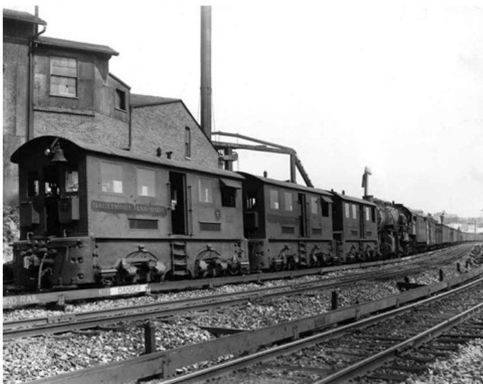
Three Baltimore & Ohio box-cab electric locomotives help a Mikado-powered freight on the Baltimore Belt Line. Four of these ungainly motors replaced the Belt Line's original steeple-cabs in 1903. Unusually, the box-cabs' four powered axles were rigidly mounted in the frame, giving them an O-D-O wheel arrangement. B&O photo.
